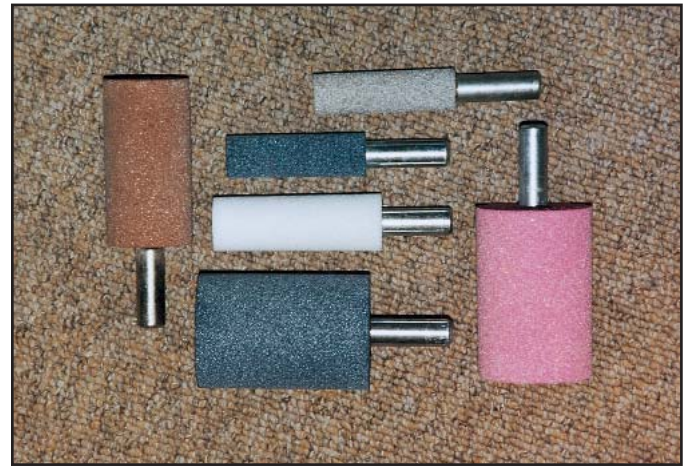
MOUNTED POINTS FOR PROFILE GRINDING MOUNTED ON 1/2" X 1-1/2 SHANKS
