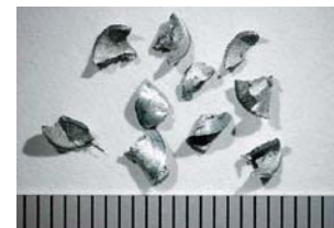
Excellent chip formation 1 scale = 1 mm
